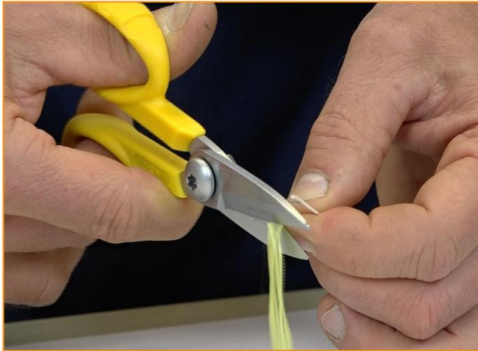
After stripping the fiber jacket, use Miller® KS-1 Fiber Optic Kevlar® Shears to cut the Kevlar® strength members in the fiber optic cables.
